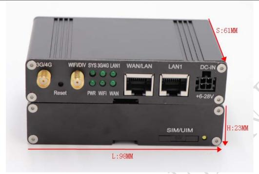
SLK-R602 is an industrial-grade high-speed wireless router based on GPRS/CDMA/WCDMA/EVDO/LTE cellular mobile network to provide users with high-speed wireless Internet and wireless data transmission functions.
