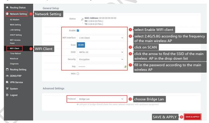
It should be noted that in this mode, the main wireless AP no longer assigns an IP address to this SLK-R680. Therefore, the obtained IP address will not be updated in "Status", and you can confirm whether the connection is successful through the icon color and MAC address. The picture below is successful.
