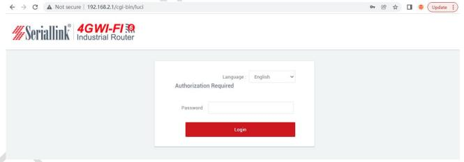
The default login password is admin. If the user needs to protect the configuration interface to avoid being modified by others, he can modify the login password, click "System" - "Modify Password" in turn, then fill in the password to be modified, and then "SAVE & APPLY", please refer to Chapter 5.3 for details.
