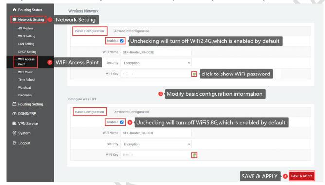
Navigation bar "Network Setting" - "WIFI Access Point" - "Advanced Configuration", under normal circumstances do not need to modify.
