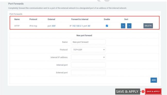
View the wan port ip, and access the internal port of the connected device or the local device through the wan port ip and external port number.
