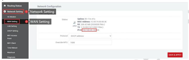
You can access the connected device directly through the IP of the wan port.(Note: The computer needs to be in the same local area network as the IP of the wan port before it can be accessed)
