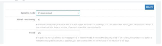
After adding and configuring, click "SAVE & APPLY" to take effect. To delete the configuration, just click the "DELETE" button in the upper right corner, and then "SAVE & APPLY".
