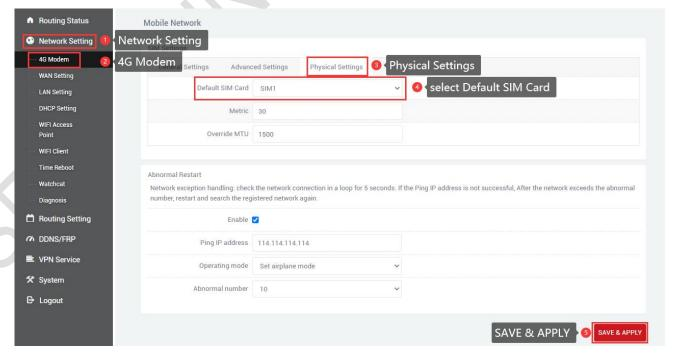
Abnormal Restart: It is to deal with network exceptions, ping the set ip address (114.114.114.114) every 5s, and still can't ping after the abnormal number of pings, it will be set according to the selection (Reboot on internet connection lost, Set airplane mode) (default), Switch SIM card). Network diagnostics can be set in "General Settings", "Advanced Settings", and "Physical Settings". You can also not enable network diagnostics, just leave it unchecked.
