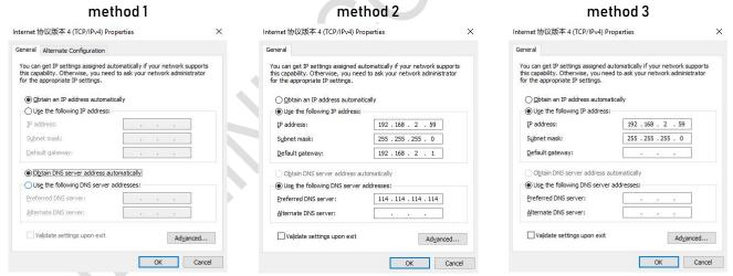
method 1: It can be used to configure the device and access the external network. It is recommended to use it (Note: If there are multiple routes with different network segments in the current environment, the IP obtained by the computer may not be able to connect to the device. In this case, method 2 can be used);
