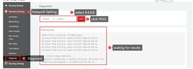
Custom input box: generally used to test whether the connected device can be pinged.
