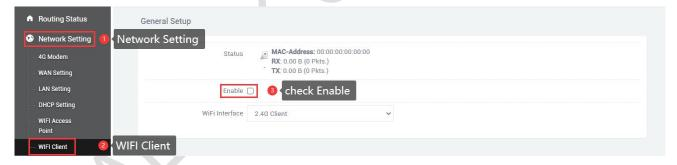
Then select the client wifi interface: 2.4G Client, 5.8G Client, search the corresponding WIFI list, select WIFI in the SSID list, change the security option according to whether there is a password, None (no password), Encryption (Encryption mixed mode Mixed WPA/WPA2-PSK), WDS is not checked by default.
