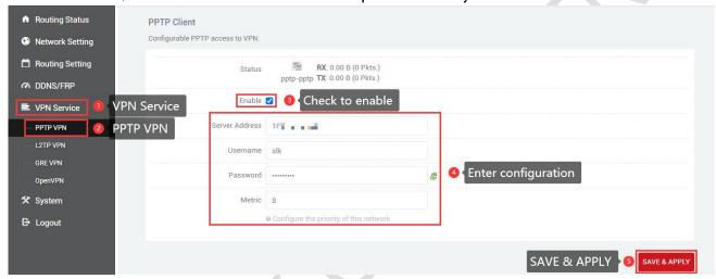
After the connection is successful, the address assigned by the server will appear in the status bar. If pptp is not used, uncheck it and click "SAVE & APPLY".
