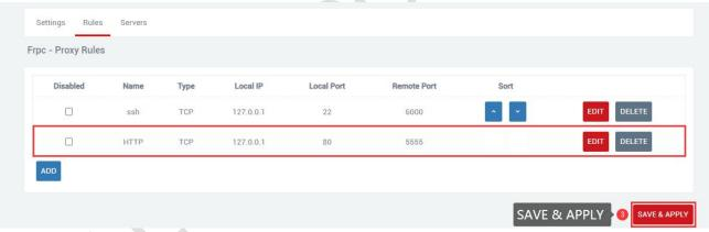
Access the local port of the local device through the public network ip and port number, and 106.107.108.109:5555 to access 192.168.2.1 (default port 80).
