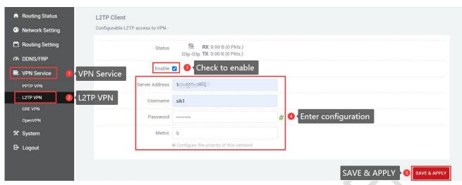
After the connection is successful, the address assigned by the server will appear in the status bar. If l2tp is not used, uncheck it and click "SAVE & APPLY".
