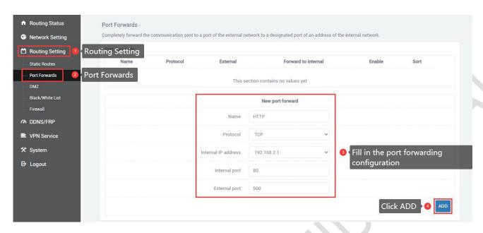
After the addition is successful, a port forwarding rule will be added. Click "SAVE & APPLY" to make the rule take effect. Multiple rules can be added.
