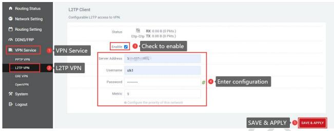
After the connection is successful, the address assigned by the server will appear in the status bar. If l2tp is not used, uncheck it and click "SAVE & APPLY".
