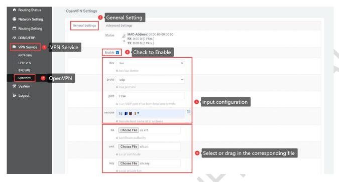
The advanced settings page is modified according to the server. If relink is checked, it means that openvpn can automatically reconnect. If you need to automatically reconnect, you can check it. If you don't need it, leave it unchecked. After all configurations are completed, click "SAVE & APPLY".
