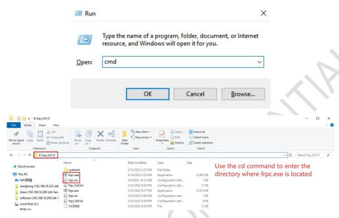
First enter "E:" to enter the disk where frpc.exe is located, then use "cd+file path" to enter the folder where frpc.exe is located, and use the command "frpc.exe -c frpc.ini" to run the client.
