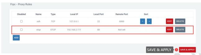
If the PC wants to access the connected device of the router as the access end, it needs to be a client of frp, and it is also the stcp protocol, but it needs to set the visitor role and bind the local address and port. The frp file for Windows can be downloaded from the company's official website. After downloading, open the frpc.ini configuration file for configuration.
